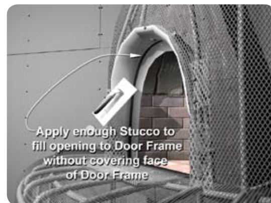
Figure 34 - Door Frame Finish
