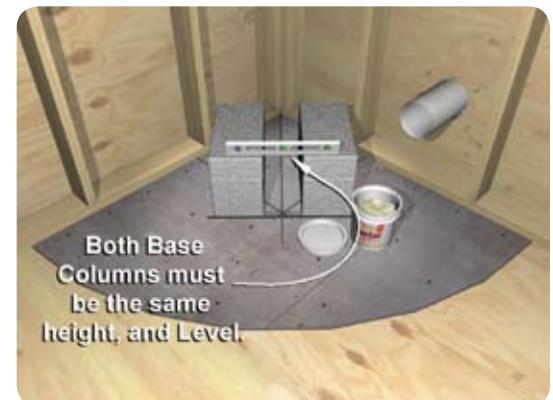
Figure 15 - Base Column Installation
