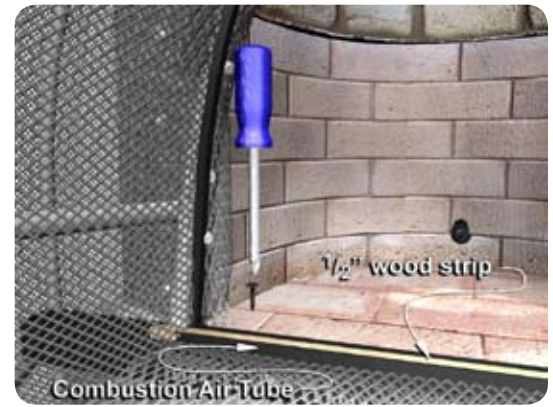
Figure 22 - Door Frame Position
