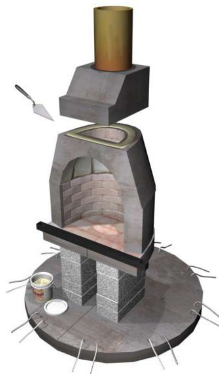
Figure 17 - Chimney Unit Installation
