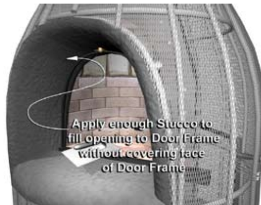
Figure 23 - Door Frame Finish
